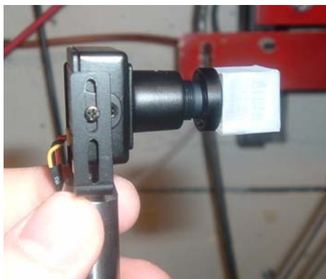
Figure 9.7 An image of a small video camera for viewing the x-ray far-field pattern. On the end of the camera is glued a block of clear Lucite (acrylic glass). On the end of the block there is a 10 \times 10 \times 0.24 \text{ mm}^3 thin cadmium tungstate crystal (see footnote 21). The camera's part number is PC212XS from Super Circuits ( www.supercircuits.com ).
