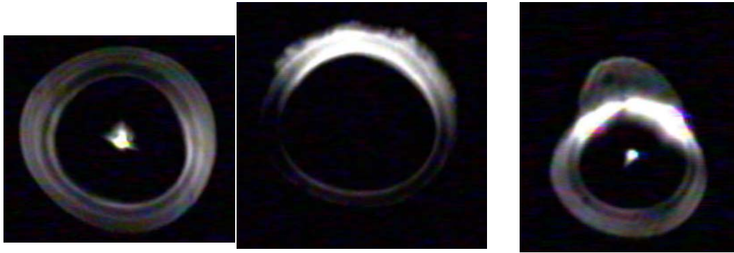
Figure 9.15 Three images showing the far-field patterns from moncapillary f1-mr9f20-02 taken at APS, beamline 18ID. The image on the left shows the entire far-field pattern (compare to f1b-mr9f20-01 in figure 4.4, an optic of the same design). The middle far-field pattern has the beam block in place. The ragged edge at the top of the far-field is due to the slightly oversized, non-ideal beam stop. The figure on the right shows the full far-field pattern after spending time in the undulator beam. Something has changed the optic's surface in that time.
