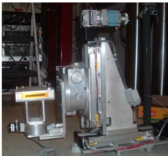
Figure C.1 An image of the x-ray transmission mirror chamber attached to G-line's GISAXS stage. The x-ray transmission mirror chamber is filled with helium to keep the transmission mirror clean in the white x-ray beam. G-line's GISAXS stage had all the motions (left-right, up-down, pitch and yaw) needed in order to correctly position the x-ray transmission mirror into the beam.
