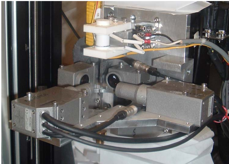
Figure B.7 An image of the two Keyence optical micrometers used to measure the glass profile both before and after the pull.
